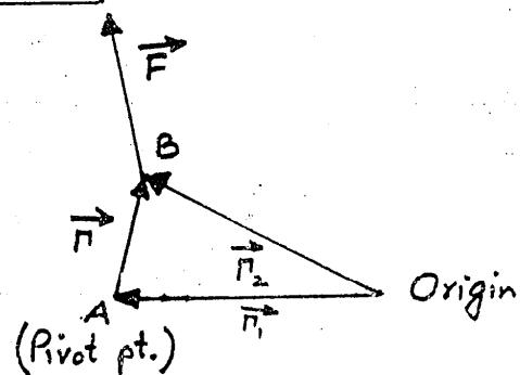
$$\vec{r}_1 + \vec{r} = \vec{r}_2 \quad \text{By head to tail rule}$$
