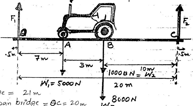
$$\begin{aligned} \text{Weight of front wheel of the tractor } W_1 &= \frac{1}{3} \times W' \\ &= \frac{1}{3} \times 15000 \\ &= 5000 \text{ N} \end{aligned}$$
