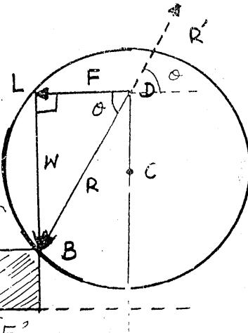
(b) - Our requirement is to calculate the resultant force 'R'. Let  $R'$  be its reactional force. In this case weight of the ball will act at point B. Two forces are acting on this ball weight and applied force 'F'.
