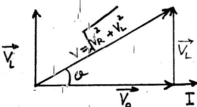
Q-16.7 A choke coil placed in series with an electric lamp in an A.C. circuit causes the lamp to become dim. Why is it so? A variable capacitor added in series in this circuit may be adjusted until the lamp glows with normal brilliance. Explain, how this is possible?
